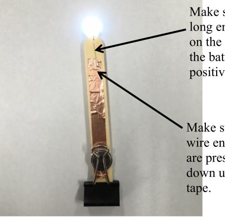
Make sure that the long end of the wire is on the same side as the battery facing positive side down.
